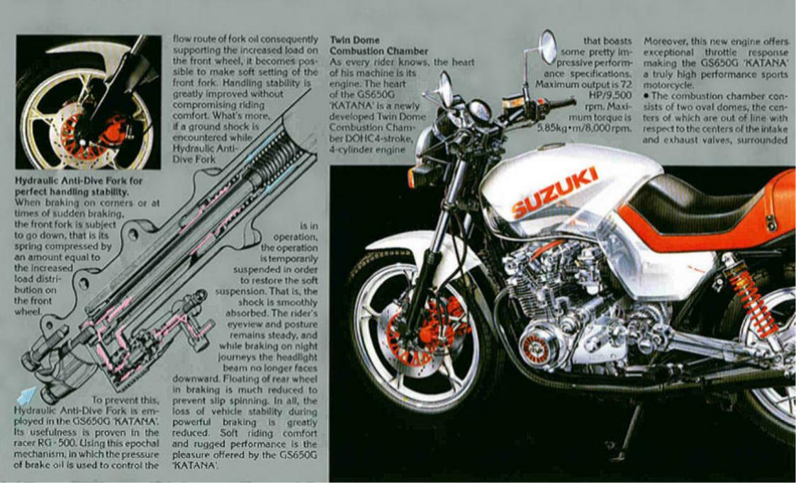
by a large conical squish zone. · Each of the two domes has an arc shaped profile that was developed after exextensive perimental test-
