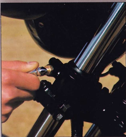
A hydraulic anti-dive fork using air/coil springs is stepless adjustable. And damping force is 4 levels adjustable.
