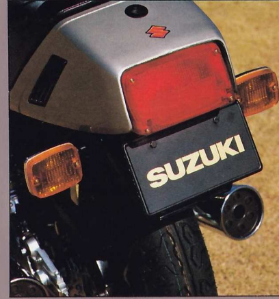
A 2-bulb tail lamp and 23 watt turn-signals provide adequate indications to other drivers.
