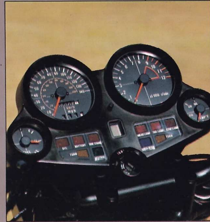
Large size speedometer and tachometer with convenient indicators for turn-signals and other indications.
