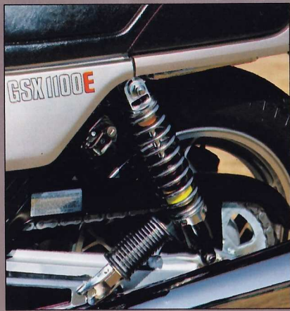
An all-round type rear suspension permits 5-stage spring preload and 4-stage damping force adjustments.
