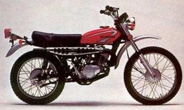
17.0 Hp at 7,000 rpm 5 speed
