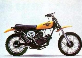
5.0 Hp at 8,500 rpm 4 speed
