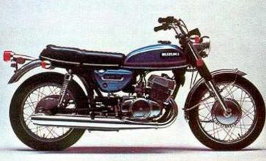
44.0 Hp at 6,000 rpm 5 speed transmission Double leading front brake Twin cylinder engine
