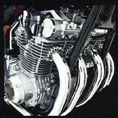
Muscular 4-stroke DOHC 4-cylinder engine powers the GS-5501, 7501, and 10001. This mighty mill uses a roller bearing crankshaft for high-RPM performance.
