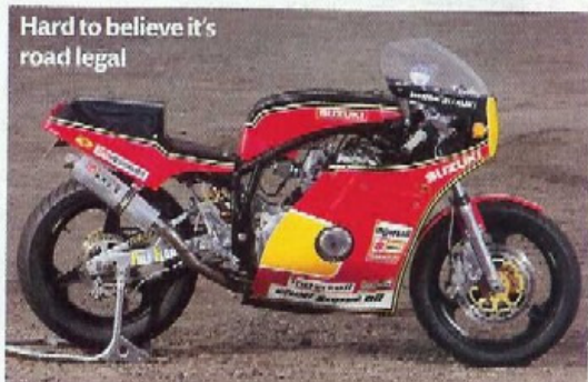
Race bike runs open ignition rotor and stainless 4-2-1 fabricated by a Northants based F1 team
